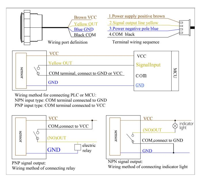
Operating principle of relay point NO output:
