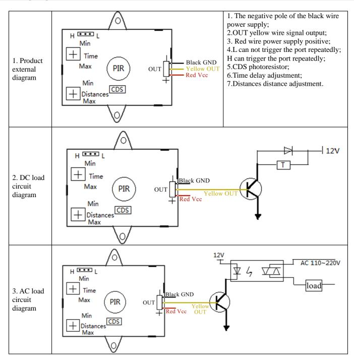
Relay normally open output (dry contact signal), that is, the relay is off when there is no induction, and the relay is closed when there is induction.
