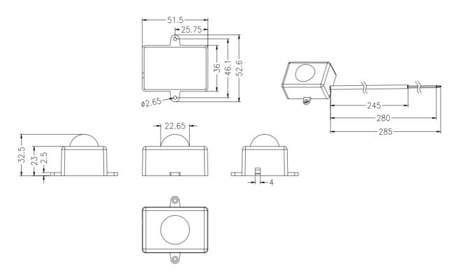
2. The following is the size drawing of model XKC-003K4-LED2A
